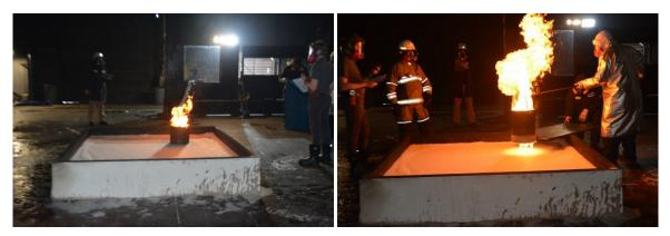
Figure 10. Start of Burnback Test (Left) and Removal of Stovepipe (Right).
