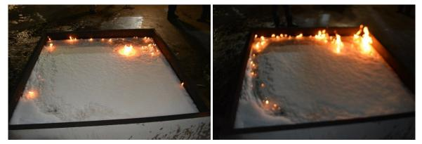
Figure 11. Initial Large Flashover Observed after Removal of Stovepipe.
