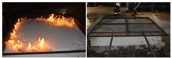
Figure 13. Largest Fire Size Observed at End of Test (Left) and Post-Test Conditions (Right).
