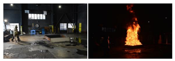
Figure 6. Pre-Test Conditions (Left) and Pre-Burn (Right) of Heptane Test Fire.
