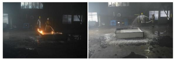
Figure 8. Foam Discharge After Control with Firefighter (Left: Small Fire, Right: Extinguished).
