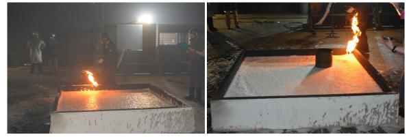
Figure 9. First Torch Pass (Left) and Second Torch Pass (Right).
