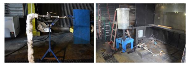
Figure 5. Special Fire Test Equipment (Left: Discharge Nozzle, Right: SwRI Pump and Tank).
