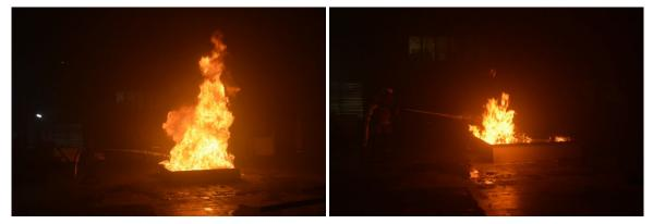
Figure 7. Foam Discharge Prior to (Left) and After (Right) Control Time.
