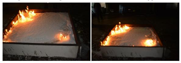
Figure 12. Additional Flame Spread During Burnback Test.
